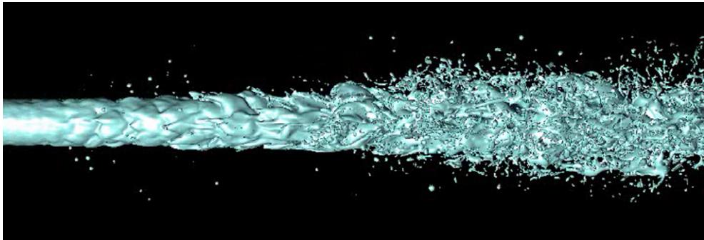
Fig. 10. Liquid jet surface and break-up near the jet nozzle.
